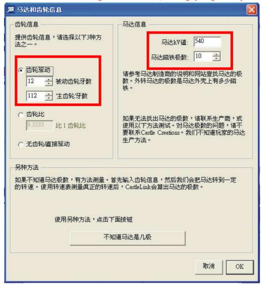
▼When using the motor on T-REX 800E, 850MX 490KVplease use 112T main gear with 12T motor pinion.
